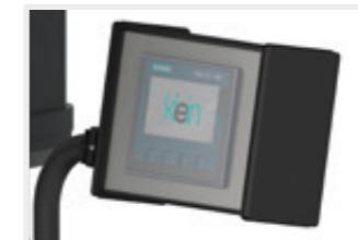
touch display for operating of spindle speed and process time
